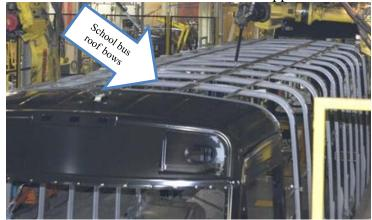
In spring 2016, while repairing a 1995 bus, the SCDE technicians saw cracks in that bus's roof bows. This led to inspection of all similar buses, some of which had been part of the 2008 structural repair.
